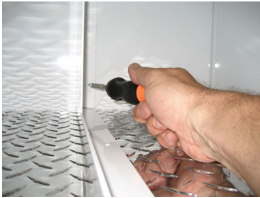
Attach floor flange and side seat flange with # 10 x 3/4" pan head sheet metal screws.
